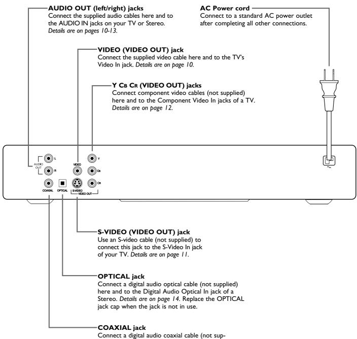
plied) here and to the Digital Audio Coaxial In jack of a Stereo. Details are on page 14.
